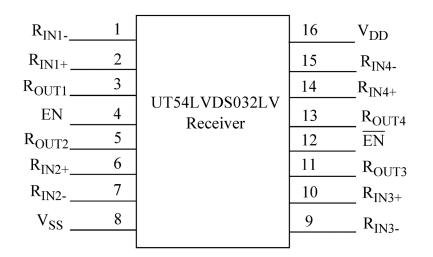
Figure 2. UT54LVDS032LV Pinout
