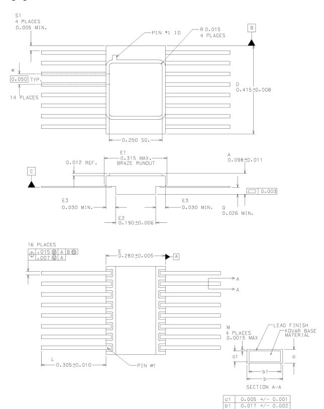
Figure 8. 16-pin Ceramic Flatpack
