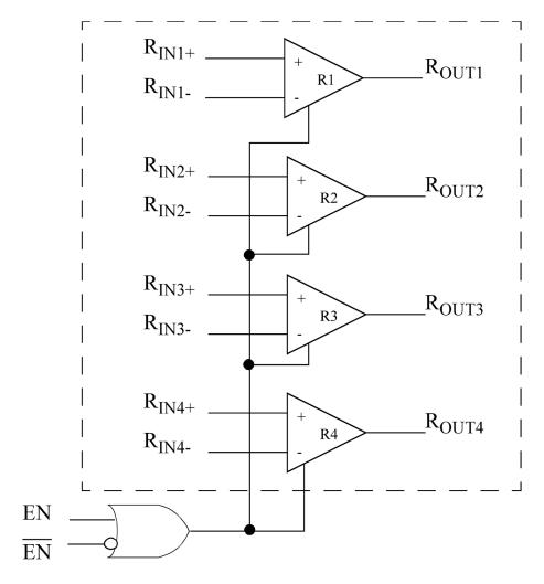
Figure 1. UT54LVDS032LV Quad Driver Block Diagram
