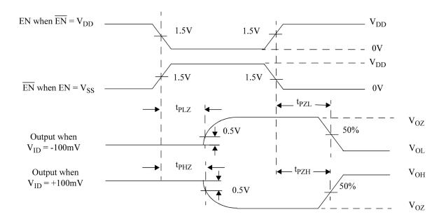
Figure 7. Receiver Three-State Delay Waveform
