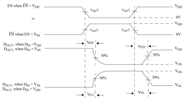
Figure 8. Driver Three-State Delay Waveform or Equivalent Circuit
