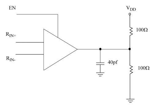
Figure 11. Receiver Three-State Delay Test Circuit or Equivalent Circuit
