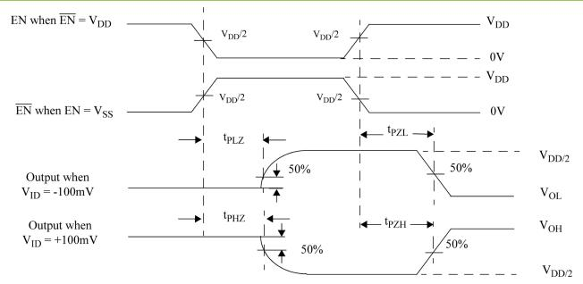
Figure 12. Receiver Three-State Delay Waveform or Equivalent Circuit
