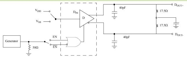
Figure 7. Driver Three-State Delay Test Circuit or Equivalent Circuit or Equivalent Circuit
