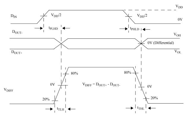
Figure 6. Driver Propagation Delay and Transition Time Waveforms or Equivalent Circuit
