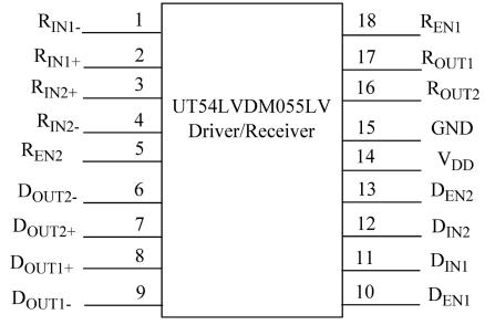
Figure 2. UT54LVDM055LV Pinout
