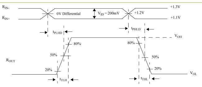
Figure 10. Receiver Propagation Delay and Transition Time Waveforms or Equivalent Circuits
